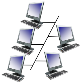
shared wire (e.g., cabled Ethernet)
